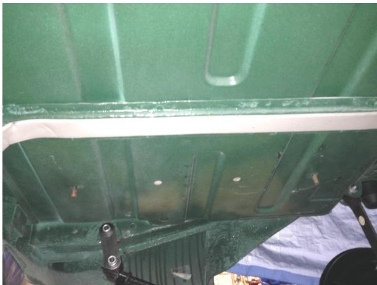
Underside of #57254 boot floor – showing rib for strap-on tank, and – in the background – studs and holes for the later bolt-on tank. Which is it?
